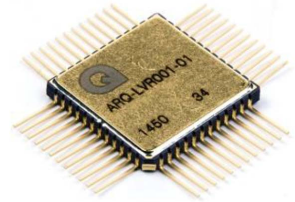
Assembled LVDS test chip of first design version ARQ-LVR001-01 in CQFP48 package
