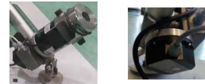
SCL is composed by two modules (actuators and observers). The SCL controller is based on PIC microcontrollers.
