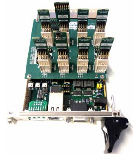
Demonstrator GR-CPCI-XC4V mounted with GR-CPCI-MEZZ-SPI-ZPACK mezzanine board
