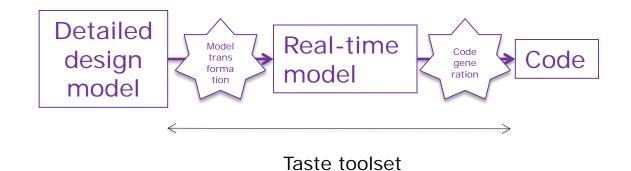
Then, from the detailed design provided by the previous step And from the behaviour of the functions provided by specific tools (Simulink. State machines) Being given the deployment view (physical topology, hardware) Taste generates the code
