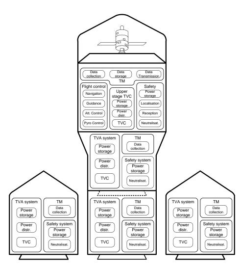
Functions to be handled by or supported by the Avionics
