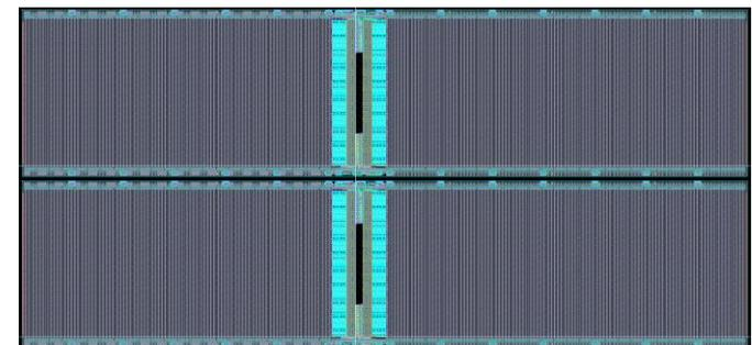
Rad Hardened High density SRAM Integration - Integrated error detection and correction. One error can be corrected and two errors can be detected, which is performed by using a (32, 7) BCH code
