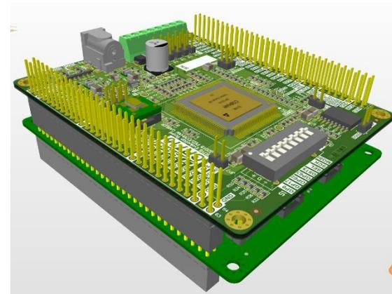
*Stack multiple boards via PC104 connector*
