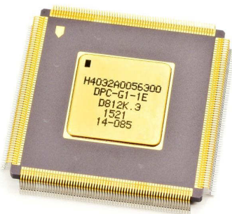
Figure 4: The qualified DPC is packaged into a ceramic quad flat pack 256 pins.
