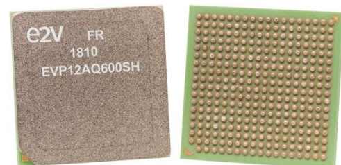
Figure 6: Top and bottom views of packaged device
