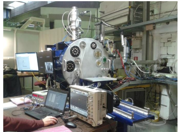
Figure 22: SEE measurement environment
