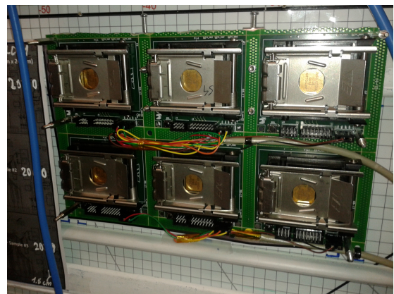
Figure 2: Photograph of the TID test PCB in the irradiation area.
