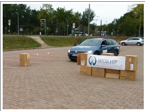
Fig. 9. Autonomous passing of a narrowing of the lane.
