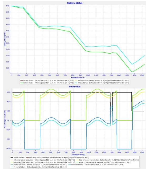
Figure 12. Battery Status (above) and Power Fluxes (below)
