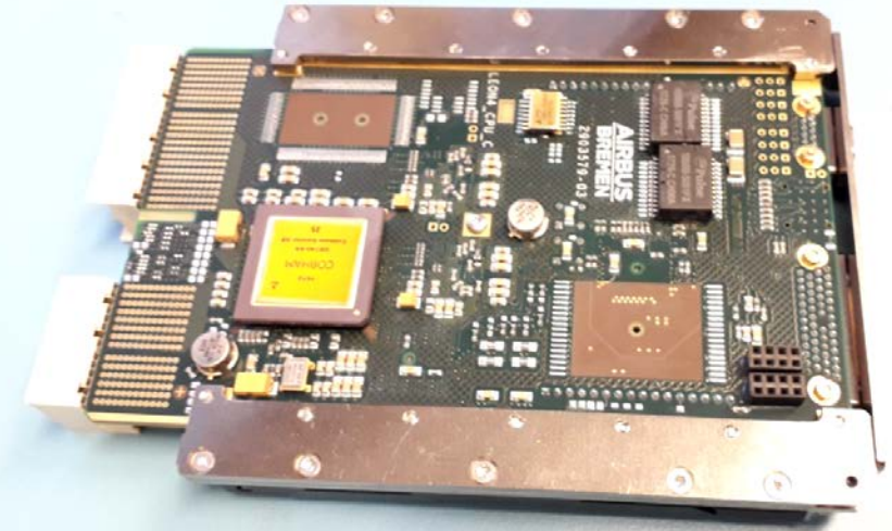
LEON4 Processor Board Bottom View
