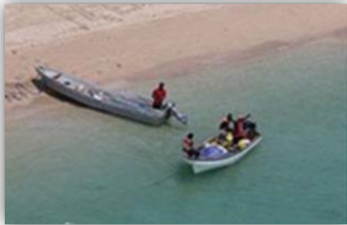
Banana Boat, Size 12-16m, Material fibre glass, Velocity 50km/h RCS M 3
