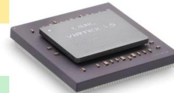
of the Virtex-52V FPGA has been qualified for high-radiation, deep-space applications.
