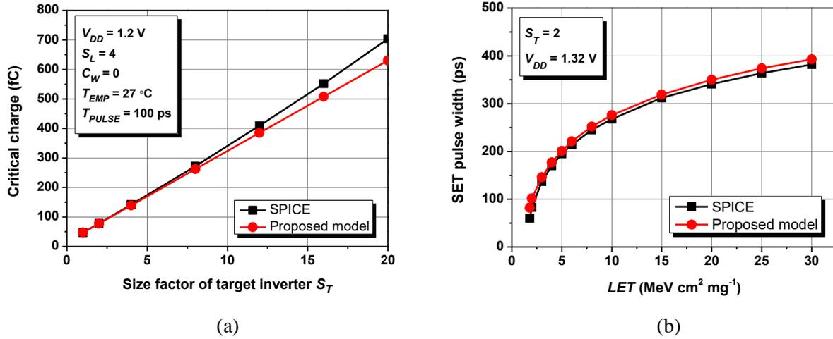
Figure 1: Comparison of proposed models with SPICE: (a) critical charge model vs. SPICE, (b) SET pulse width model vs. SPICE
