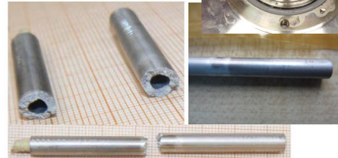
Figure 3: ATJ AA2219-AA6082 S/N 07, after tensile testing, supporting pin jammed in the clamping area
