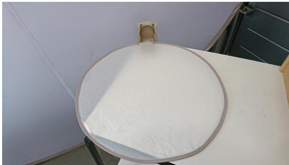
Dragsail subsystem with the unfolded/deployed sail
