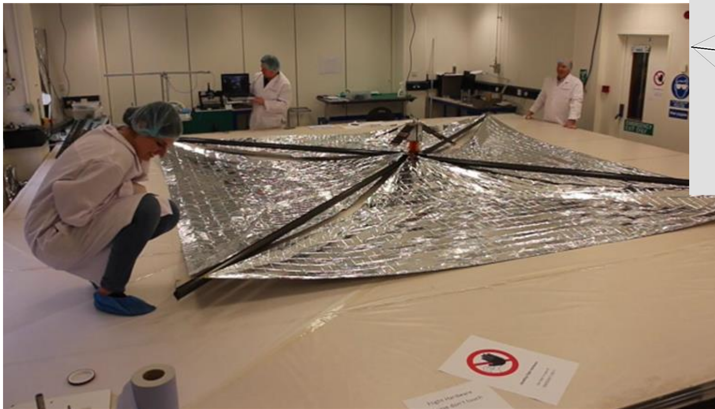
Unfolded Rigid Boom Electro-Dynamic Drag Sail (RBEDDS)
