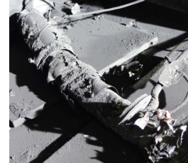
Overcharge at 2C - SOC at CID activation
