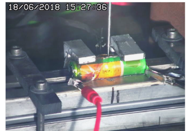
Nail test on a HC cell Release of smoke
