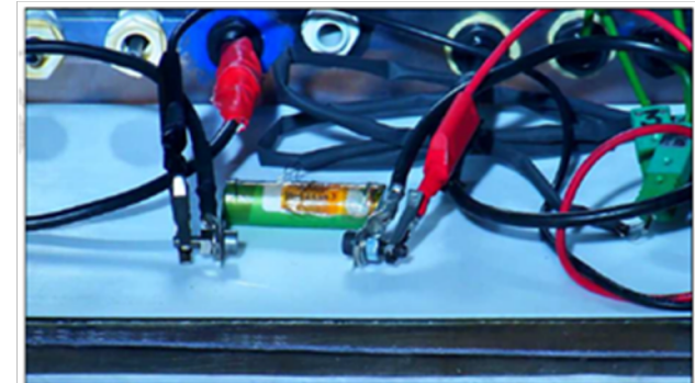
100 mΩ short-circuit on HCM cell
