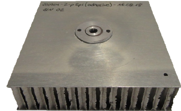
2 part Insert sample with adhesive technology
