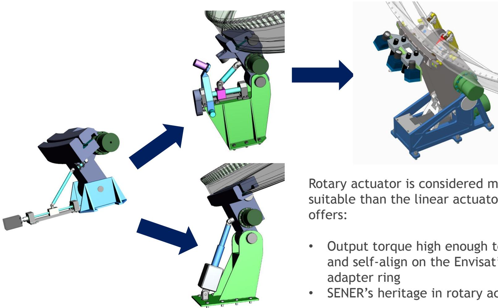
Rotary actuator is considered more suitable than the linear actuator as it offers:
