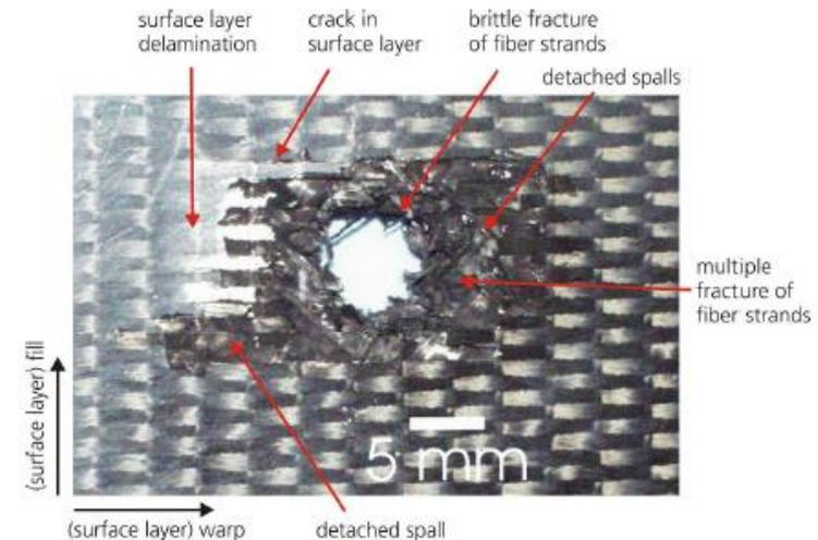
Example - debris damage due to 3 mm Al-sphere at 4550 m/s
