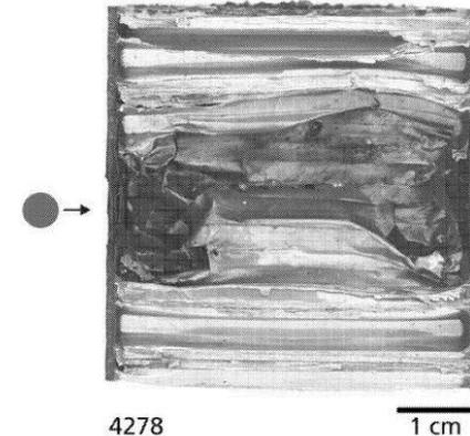
Example - debris damage due to 3 mm Al-sphere at 4490 m/s
