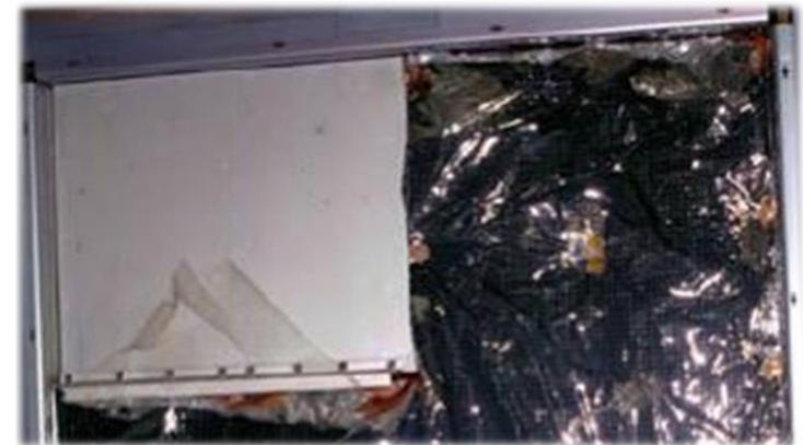
Pre and post-flight pictures of the radiator panel covered with the silvered Teflon coating
