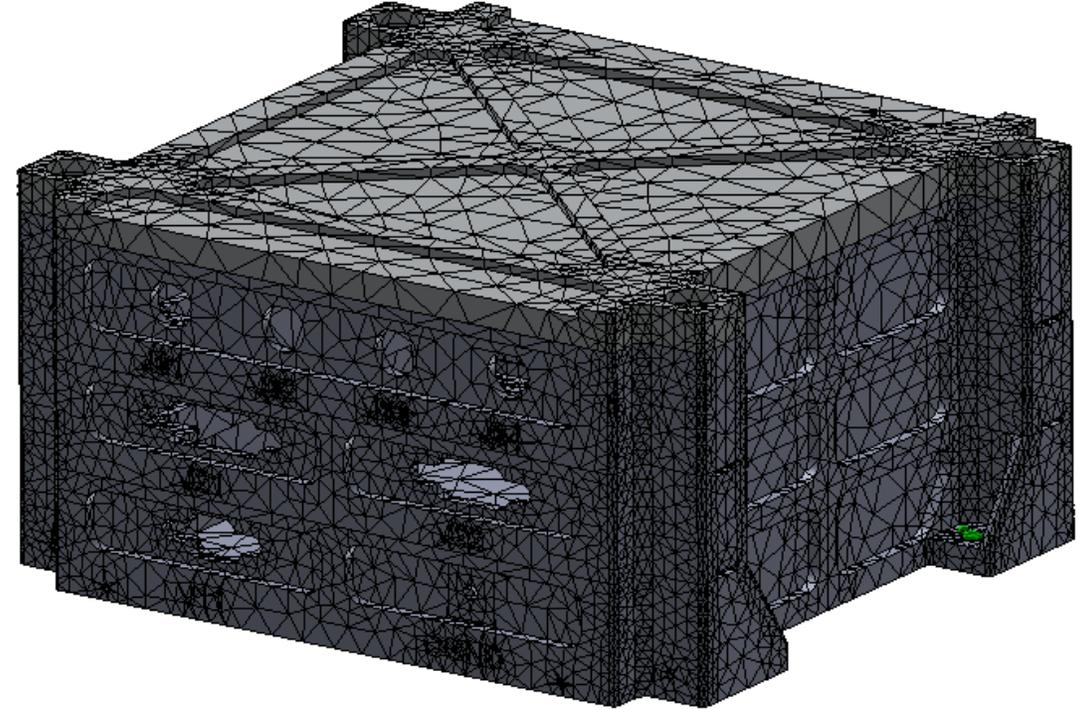
Modal analysis and dynamic analysis conducted using SolidWorks
