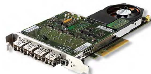
Napatech NT4E2-4-PTP Ethernet Interface Board
