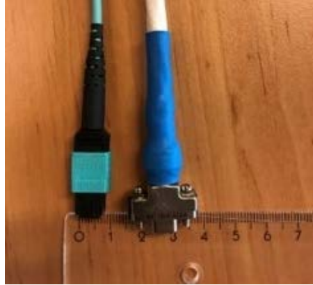
Harness diameter 12 Fibre 60 Gbps (6x10 Gbps) vs single SpW cable (200 Mbps)
