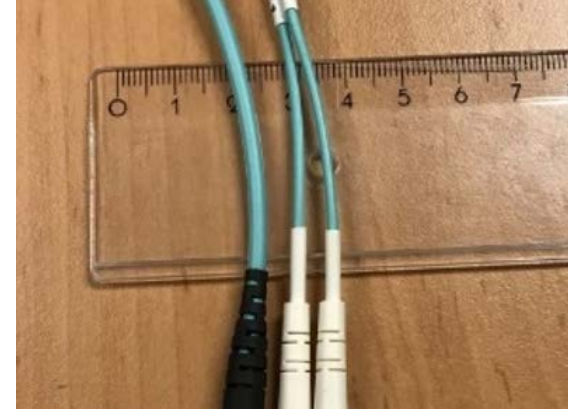
Harness scalability Single vs 12 fibre cable – scales nicely
