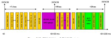
Figure 5-29: EDM CAN bus B TM/CMD window
