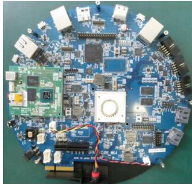
The outlook of Space Cube® mk4 and its interior assembly
