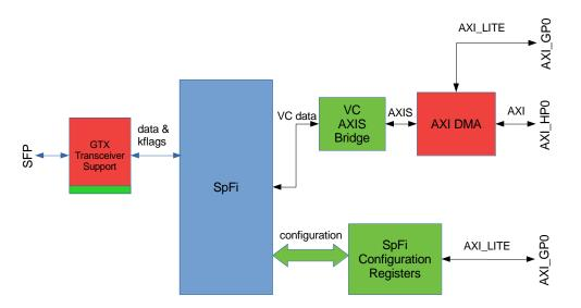
Colour legend: blue: ESA IP core red: Xilinx IP core green: ITTI IP core red+green: generated by ITTI based on Xilinx templates
