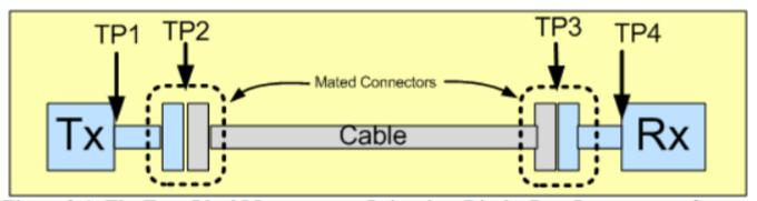
Figure 2-1: The Four Ideal Measurement Points in a DisplayPort Interconnect System
