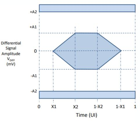
Figure 5-12: Serial eye pattern mask
