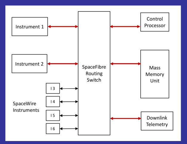
SpaceFibre links carries SpaceWire packets with much more functionality:
