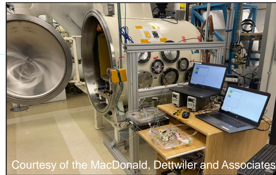
Figure 11. TVAC Testing Chamber and Test Station
