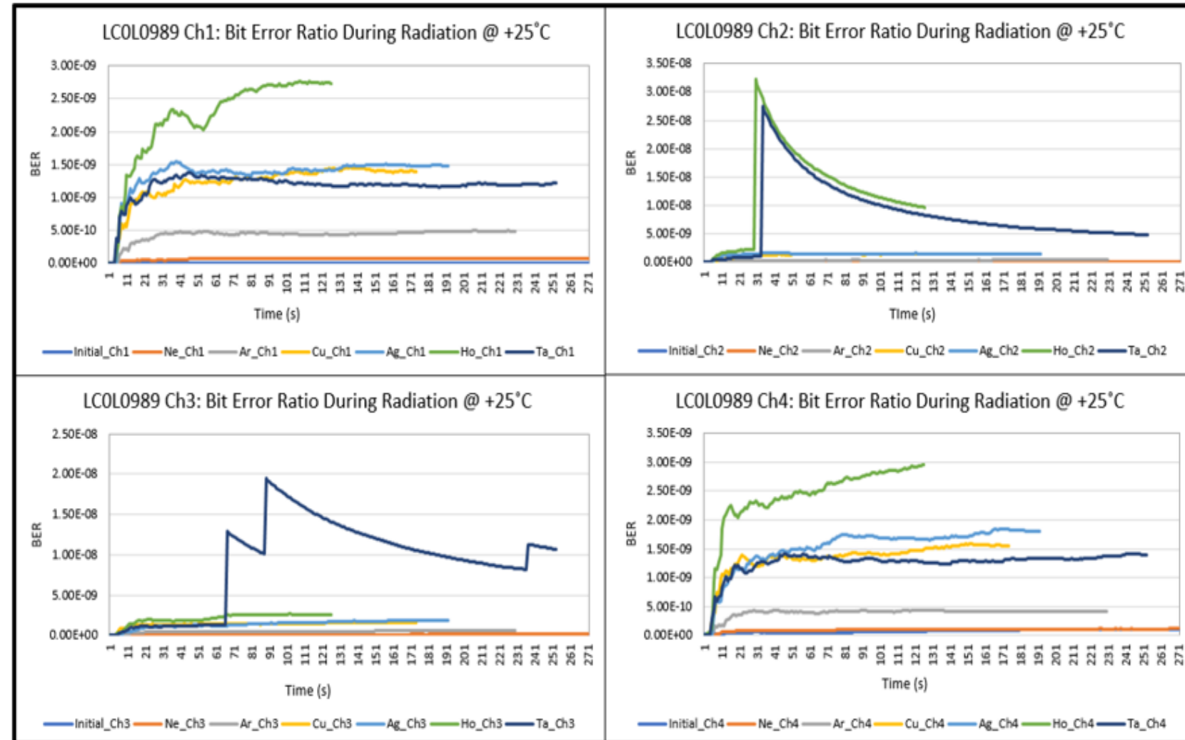
Fig. 6. Transceiver BER Monitoring Under Heavy Ions Radiation
