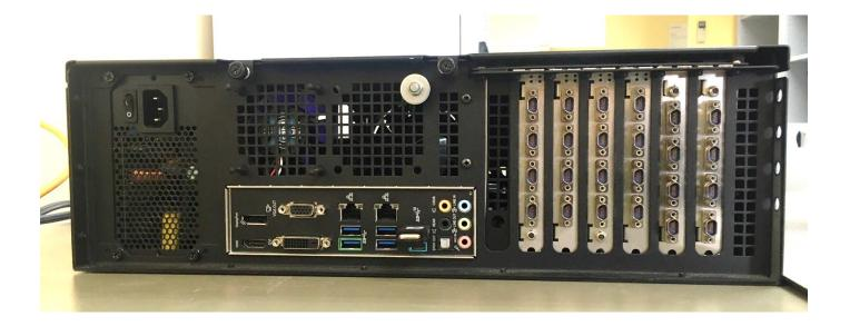
Two iSAFT quad SpW cards Simulating the SpW Nodes
