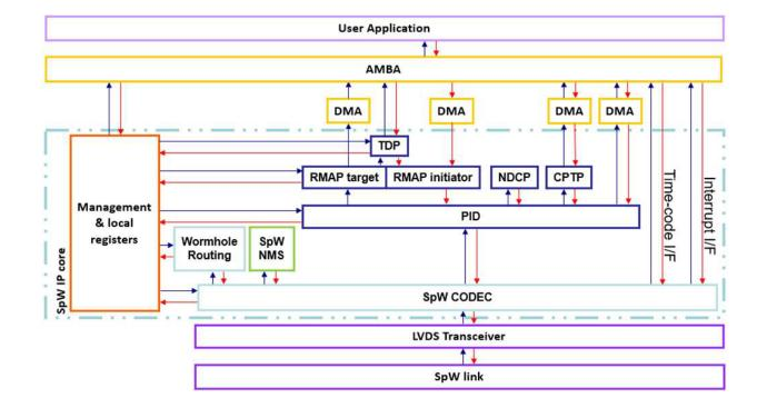
Proposed SpW NMS block can replace traditional Wormhole routing implementing a Store and Forward approach with ingress policing, packet filtering and traffic shaping
