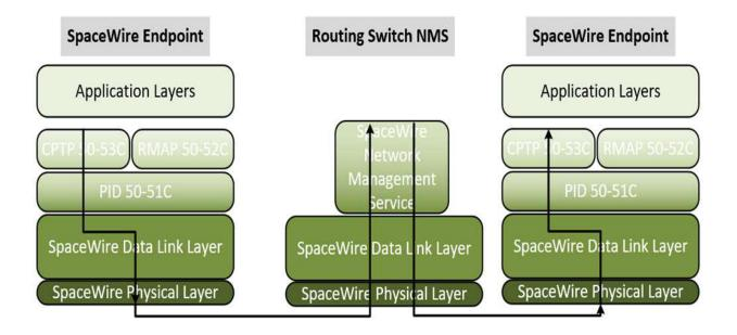
Analysis on the new protocol determines that the SpW node shall not be modified in order to retain compatibility with all existing SpW units. All new functions will be implemented in the SpW Switch level.
