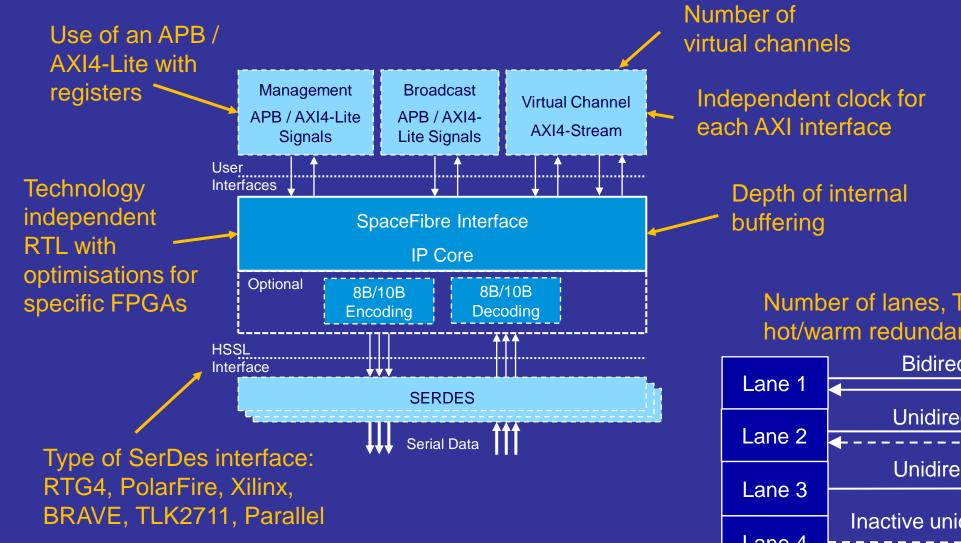
Number of lanes, Tx/Rx unidirectional lanes, hot/warm redundancy
