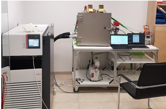
Figure 1: TVC Thermal vacuum chamber testbench
