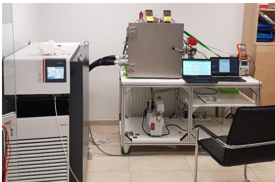
Figure 1: TVC Thermal vacuum chamber testbench
