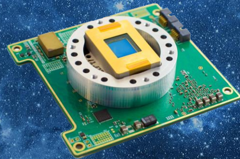
NANOimager Miniaturized multispectral SWIR imager (ACQ unit)
