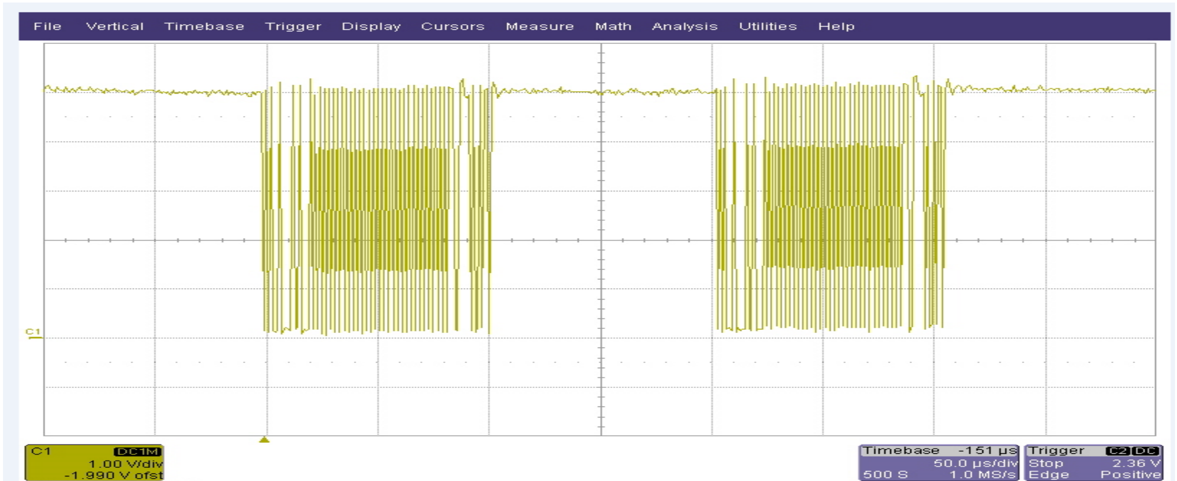
Figure 2: Scope plot of two data packets
