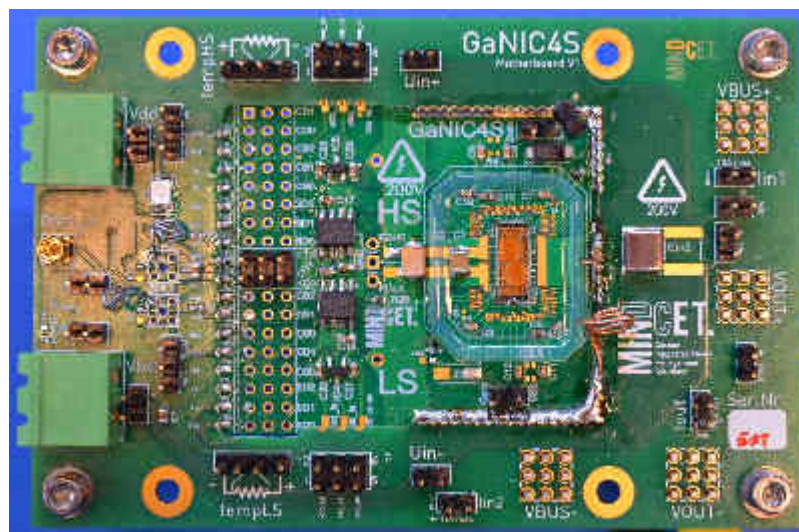
Figure 3 10A point of load converter using integrated GaN ½ bridge
