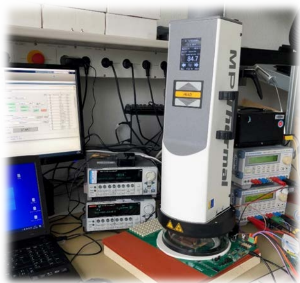
Figure 4: Screening tests: electrical measurement over temperature at IMST
