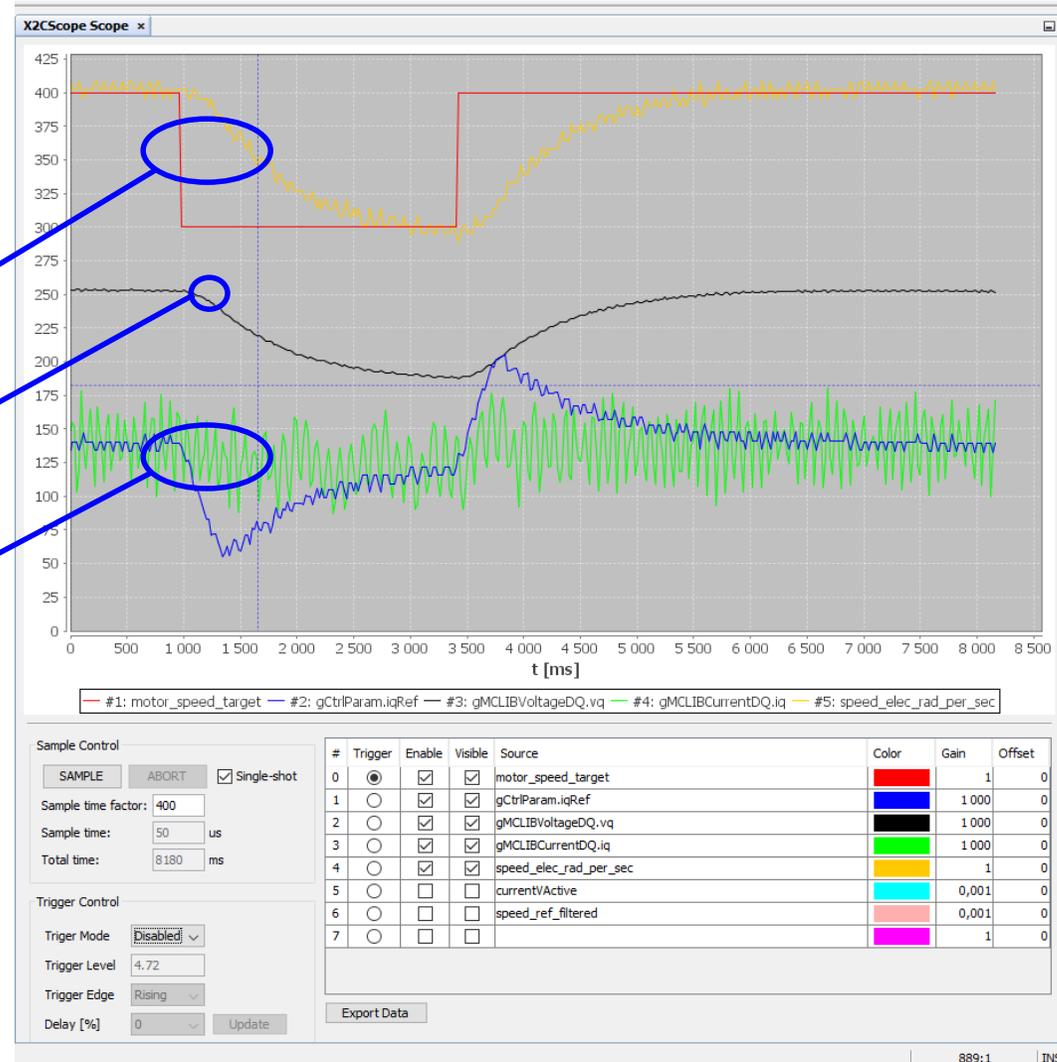
Note: Ripple in the current target (green) is due to the asymmetric torque in the load.
