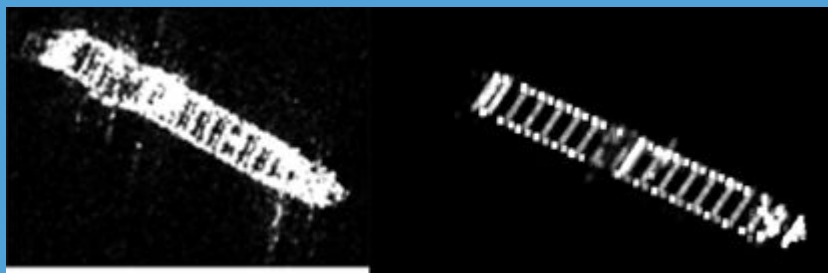
CONTAINER SHIP (LEFT: TERRASAR-X IMAGE, RIGHT: SIMULATED SIGNATURE) - 0,9M X 1,8M PIXEL SPACING
