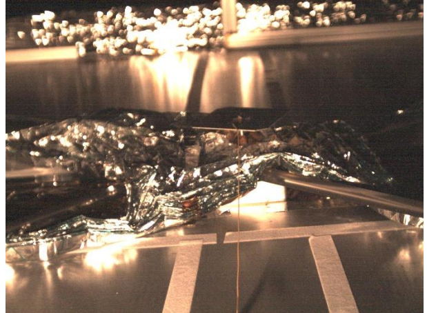
Figure 7: Thermal-vacuum deployment (hot case 70°C). The picture shows ADEO-N just after a successful deployment under thermal-vacuum conditions in DLR's Space Simulation Chamber. Note, that a full deployment without gravity compensation and within the chamber is not possible.
