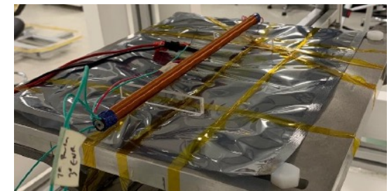
Proof of concept of short-circuit triggering system (left) and short-circuited magnetorquer (right)
