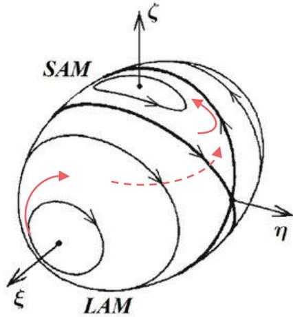
Angular rates in body principal axes for a given angular momentum  $H$
