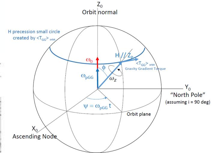
*Precession motion of the angular momentum around the orbit normal due to Gravity Gradient*
