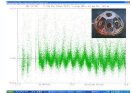
Fig. 5: Each of the 8 retros of the ENVISAT reflector unit slightly changes its distance from the SLR station, as ENVISAT is rotating; 8 'peaks' thus correspond to ONE full rotation of ENVISAT
