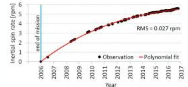
The history of T/P inertial spin rate: SLR and photometric data combined.
