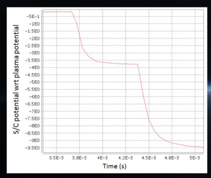
S/C potential wrt plasma potential when 6 V and 13 V steps applied to the probe
