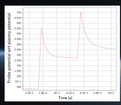
Probe potential wrt plasma potential when 6 V and 13 V steps applied to the probe
