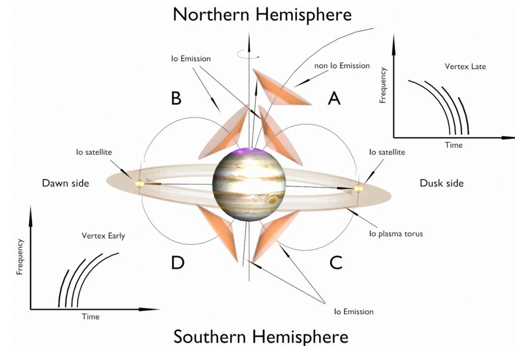
**Figure 1:** Location of the beaming cones of the different components of the jovian satellite-induced radio emissions detected by an observer. The location is defined with regard to the observer position, which is out of the figure plane in the example. The emissions' dominant polarization indicates the hemisphere of origin and their arc pattern on dynamic spectra, the side of the source location. From Marques et al., 2017.
