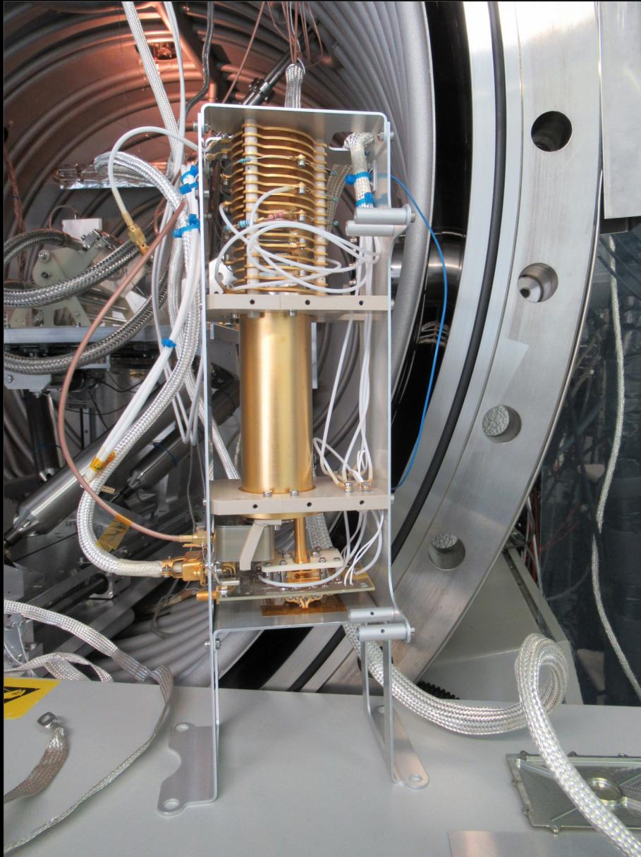
We have built a new time-of-flight mass spectrometer for ice experiments in house: faster, more sensitive, and higher mass resolution than old QMS.
