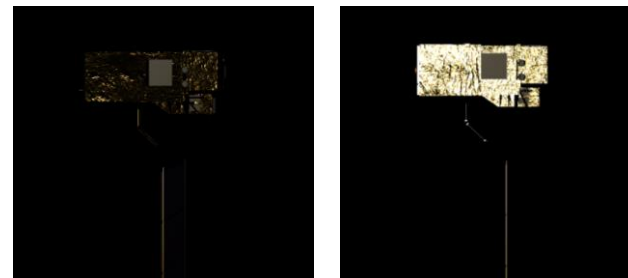
Impact of the illumination on Sentinel-3 model (20deg delta), mainly specular
