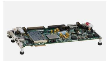
Embedded processing system with programmable logic based on Zync-7000 XC7Z045 SoC
