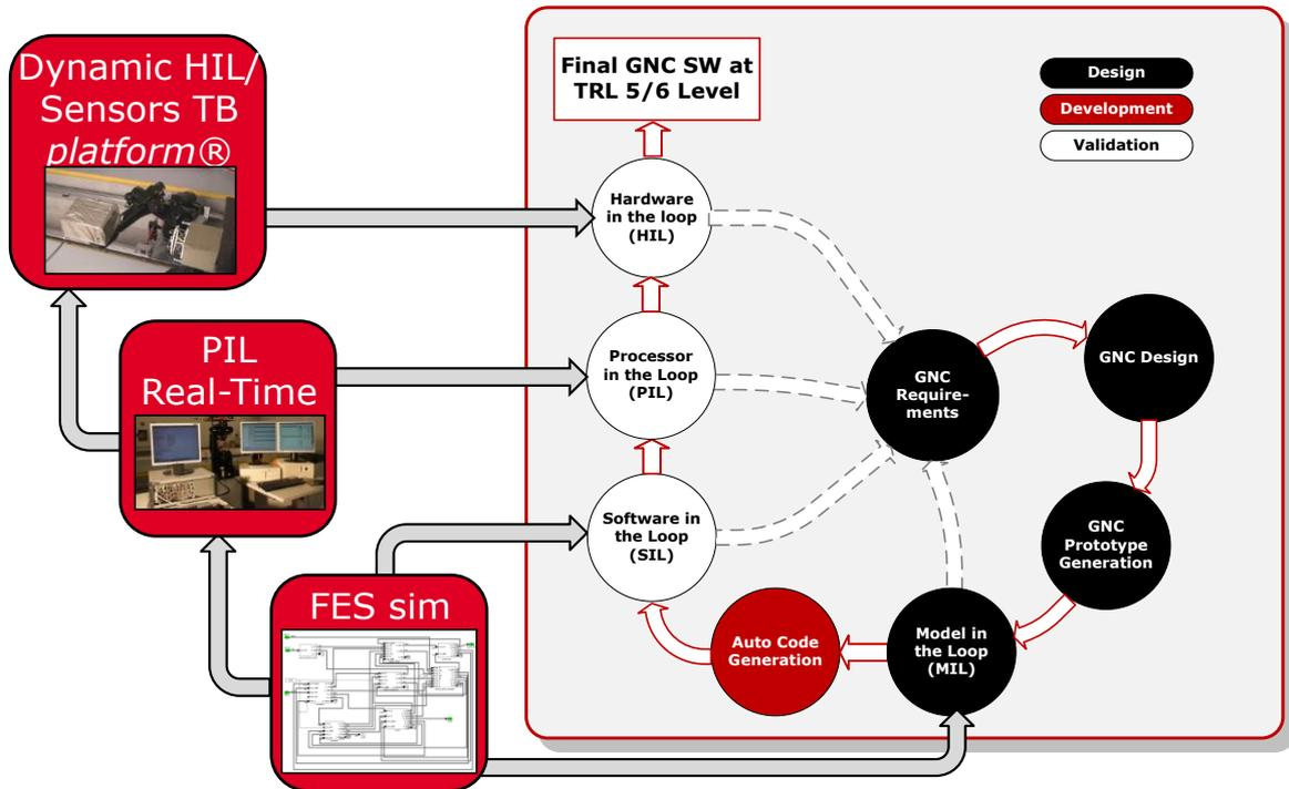
**Figure 1. Coherent, incremental, highly automated GNC Design, Development, Verification and Validation (DDVV) Approach.**
