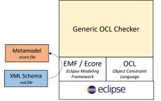
First level of the OCLChecker tool corresponds to the generic features to automate OCL checks, manage OCL rules by rulesets, produce result through the Eclipse GUI and also in batch mode. This first level is generic and is not linked to any OCL rule nor domain model.
