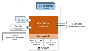
This generic tool is instantiated by each software provider with its dedicated meta-model(s) and OCL rules, enabling domainoriented evaluation of constraints and consistency checks.
