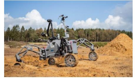
SherpaTT during the field tests of the ADE demonstrator developed with TASTE (Courtesy of DFKI)
